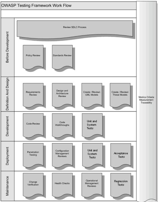
Figure 5: Typical SDLC Testing Workflow.
